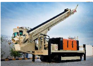
Blast hole drilling
