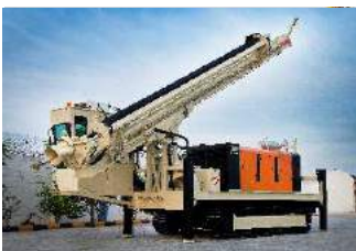
Blast hole drilling
